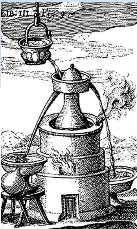
Alambic with water cooling around the distillation helmet.
